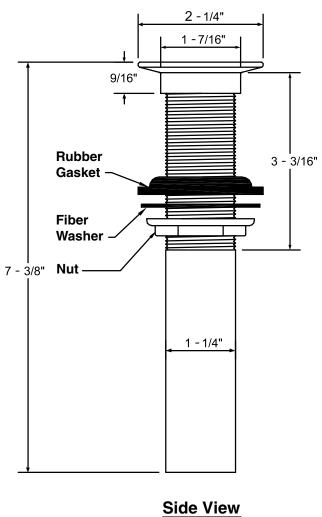
Model: D4500 1 1/4" Grid Strainer without overflow
