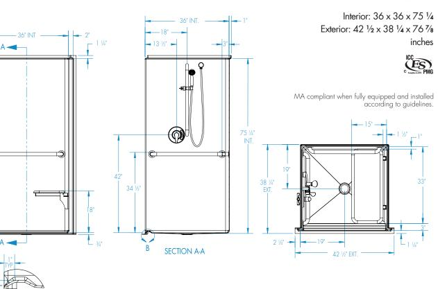
FEATURES Dimensional Tolerance ± 36". Dimensions needed for site preparation should be measured from the unit. Aquatic assumes no responsibility for preparatory work.
