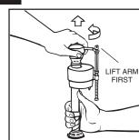
IMPORTANT: Always clear sand and rust from system. • Make sure water supply is off. Remove valve TOP by lifting arm and rotating top and arm 1/8 turn counterclockwise, pressing down slightly on cap.  While holding a container over the uncapped VALVE to prevent splashing, turn water supply on and off a few times. Leave water
