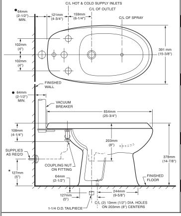
The bidet is not furnished with a trap. Provisions must be made for the installation of a trap in the floor.
