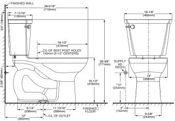
NOTES: THIS TOILET IS DESIGNED TO ROUGH-IN AT A MINIMUM DIMENSION OF 305MM (12") FROM FINISHED WALL TO C/L OF OUTLET.
