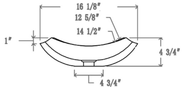
Dimensions of fixture are nominal and may vary within the range of tolerances established by ASME Standard A112.19.2. Dimensions and specifications subject to change without notice.
