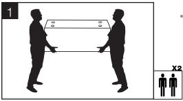
• The acrylic bathtub must be carried in an upside-down position. It must never be carried by its acrylic panels. Two persons required.
