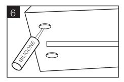
• Apply silicone to the feet of the bathtub that stands on the floor.
