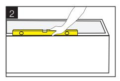
The bathtub is leveled via a water level at the intended local installation area.
