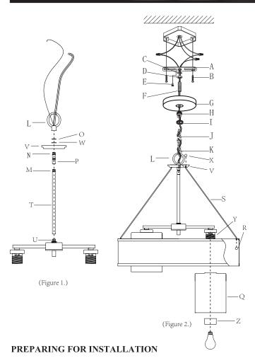
Remove all contents from the carton. See the important notes above. Shut off the power at the circuit breaker and completely remove the old fixture from the ceiling, including the old mounting bracket.
