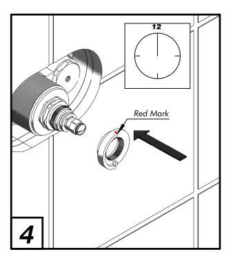
STEP THREE once you have the temperature set correctly, remove the plastic guide by pulling it towards you. You will notice a red mark on the guide. Reinstall the guide with the red mark pointing to the twelve o'clock positions. This will indicate the correct setting for your valve to function at the dialed setting indicated.
