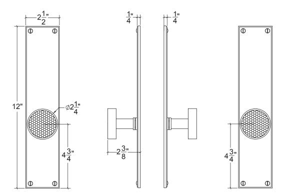
**Mortise Lock** standard backsets are 2-1/2" and 2-3/4" **Tubular Latch** standard backsets are 2-3/8" and 2-3/4" Can work with 2-1/8" face bores
