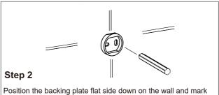
Position the backing plate flat side down on the wall and mark holes with pencil.
