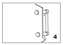
Fix the set screws on the handle, tighten it to avoid loose from fixing brackets.
