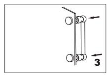
Add the handle A on the fixing brackets, make sure the set screws holes in the bottom.
