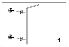
Install the end cap "4" (bolt) through the glass holes,make sure the rubber gaskets are between handle&glass.
