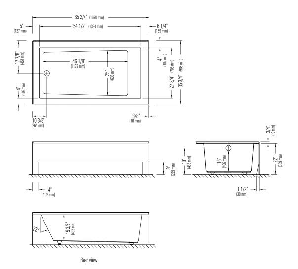
\*A bathtub fitted with back jets can cause the pump to protrude
