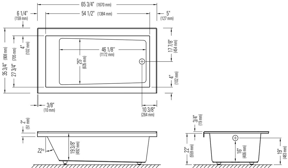
\*A bathtub fitted with back jets can cause the pump to protrude by approximately 3" from the overall dimension.
