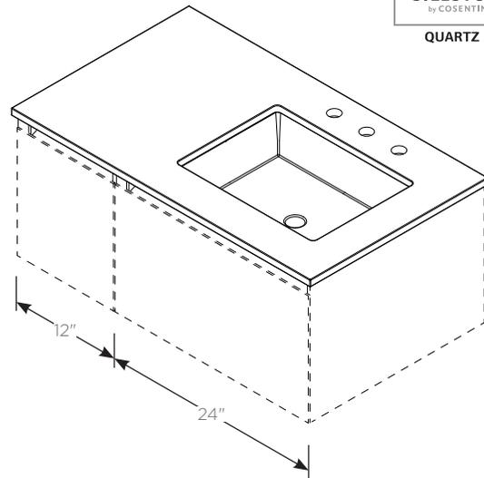
**Note:** Sinks must be located over H1-Tip Out or H2/V14 Plumbing drawers. See Cartesian Reference Guide for more information.
