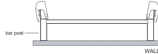
2. Using the Allen key provided, remove the mounting posts from the bar posts. Press the mounting posts against the bar post flange positions on the wall and mark the screw hole positions.
