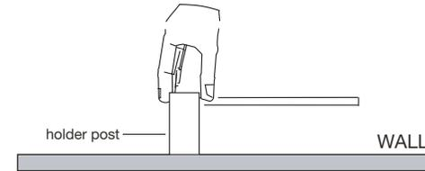
2. Using the Allen key provided, remove the holder post from the mounting post. Press the mounting post against marked post position on the wall and mark the screw hole positions.
