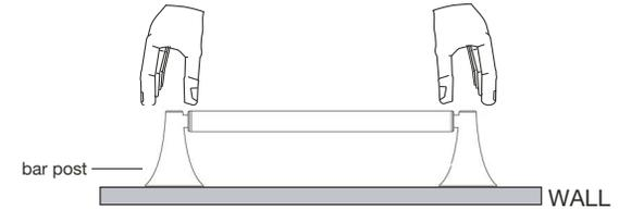
2. Using the Allen key provided, remove the holder post from the mounting post. Press the mounting post against marked post position on the wall and mark the screw hole positions.
