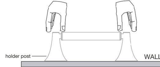
2. Using the Allen key provided, remove the holder post from the mounting post. Press the mounting post against marked post position on the wall and mark the screw hole positions.
