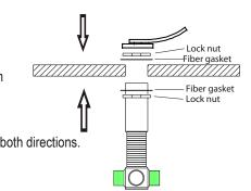
\*\* The spout, handle valve bodies and diverter can be connected with flex hoses (not provided by Santec) or copper pipe soldering. Please note that when soldering connections, do not use excessive heat. Excessive heat can damage the joints increasing probability of leakage.
